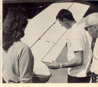
scratches. The Floes look for loose hinges or worn pins. (5) TRIM TABS. The trim tabs, like the ailerons, should be checked for snugness. Look here, too, for loose rivets or torn fabric. (6) LANDING GEAR. Any airplane with a retractable landing gear should be put on a hoist so that gear retraction can be tested; fairing doors should close completely. (7) NOSE WHEEL. There
